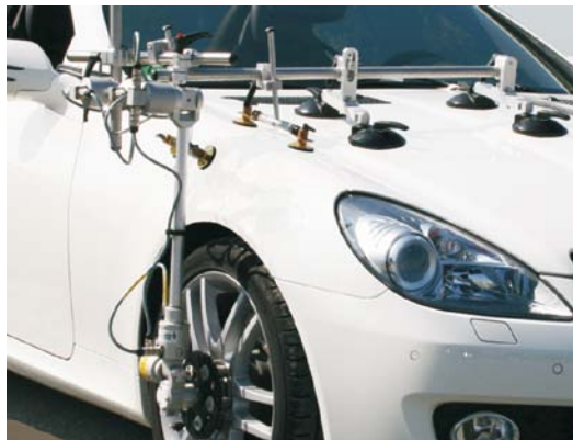
Fig. 3: RV-4 sensor, front wheel mounting with 4-point suction holder
