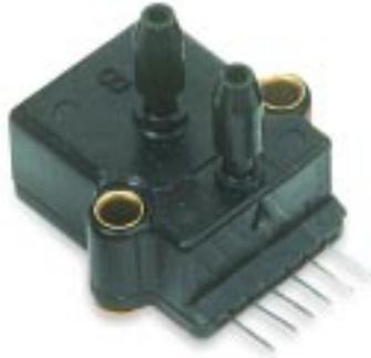
The SCX series sensors provides a very cost effective solution for pressure applications that require high accuracy over a wide temperature range. These internally calibrated and temperature compensated sensors were specifically designed to provide an accurate and stable output over a 0°C to 70°C temperature range. This series is intended for use with non-corrosive, non-ionic working fluids such as air, dry gases and the like.
