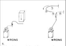
Limit switches are designed for proper performance with the actuators with which they are supplied. Supplementary actuators should not be used unless the limit switches are specifically designed for them.
