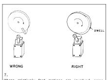
Where relatively fast motions are involved, cams should be designed such that the limit switch will be held operated long enough to operate relays, valves,
