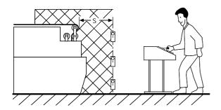
The number of beams to be used needs to be defined according to the risk assessment and to the probability for the machine operator to bypass the protection. Particularly, during risk assessment, methods of defeating safety equipment shall be taken into account before selecting the correct configuration.
