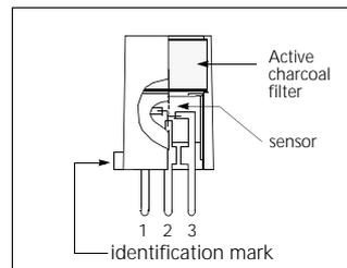
Fig 1c. Pin Layout
