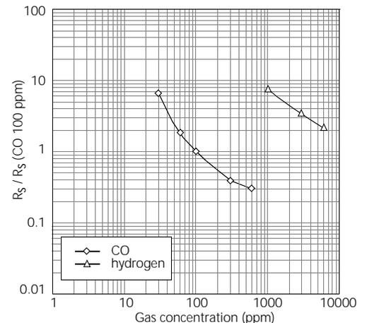
Fig 3b. SB-95-12: Sensitivity at LOW signal for CO
