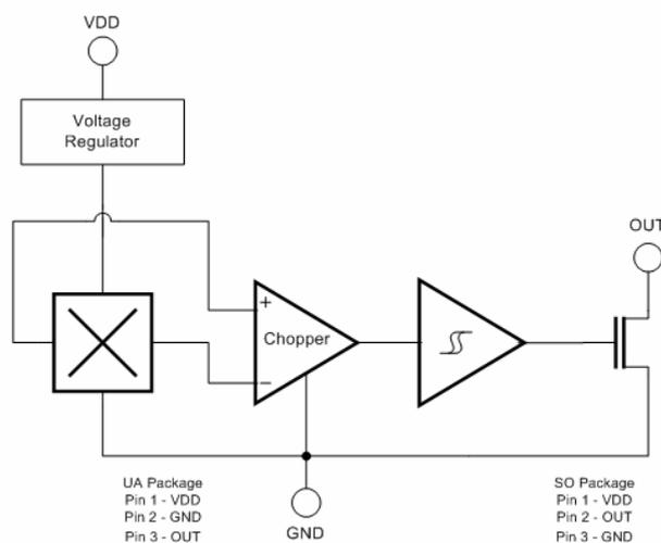
**Note:** This is a static-sensitive device. Please observe ESD precautions. Reverse VDD protection is not included. For reverse voltage protection a 100Ohms resistor in series with VDD is recommended.
