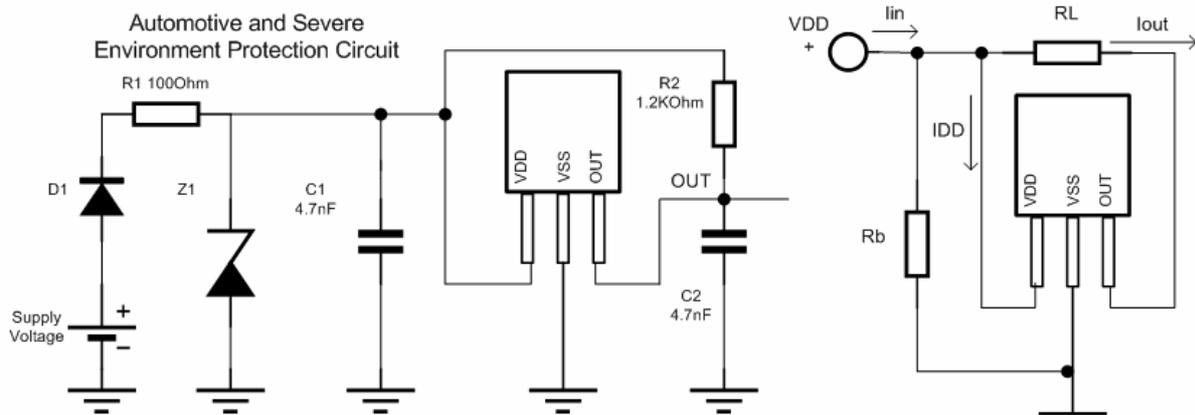
The resistors RL and Rb can be used to bias the input current. Refer to the part specifications for limiting values. This circuit will help in getting the precise ON and OFF currents desired.
