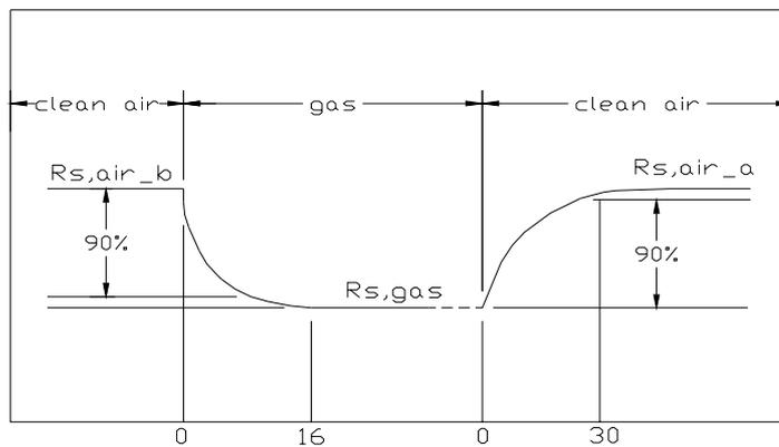
$R_{s,air\_b}$  : before injecting gas, resistance in Clean Air Condition
