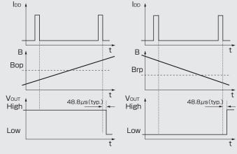
Releasing Point Timing Operating Point Timing
