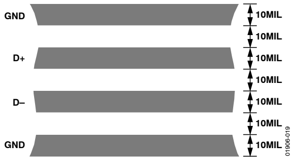
Figure 19. Arrangement of Signal Tracks
