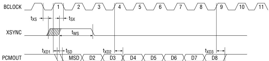
When  $t_{XS} \leq 1/2 \cdot F_c$ , the Delay of the MSD bit is defined as  $t_{XD1}$ .
