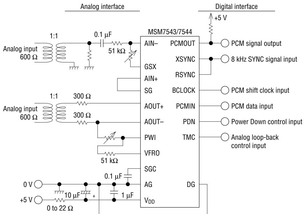
**FREQUENCY CHARACTERISTICS ADJUSTMENT CIRCUIT**
