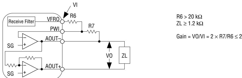
During power saving and power down modes, the outputs of AOUT+ and AOUT- are in a high impedance state .
