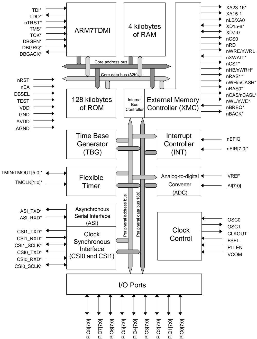
Asterisks indicate signals that are secondary functions of I/O ports.
