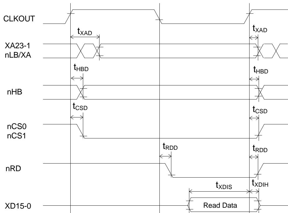
Bank 2 and Bank 3 Read/Write Cycle Timing
