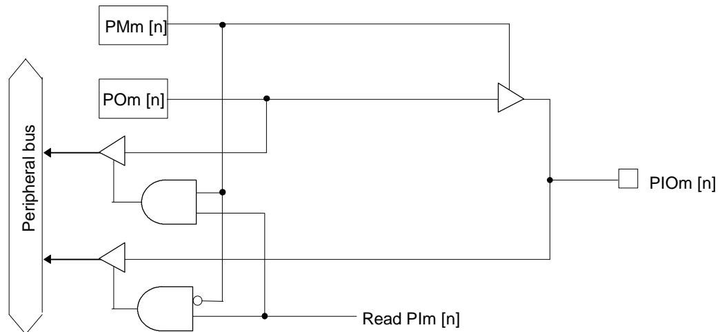
○ I/O port B (I/O ports with second functions of input)
